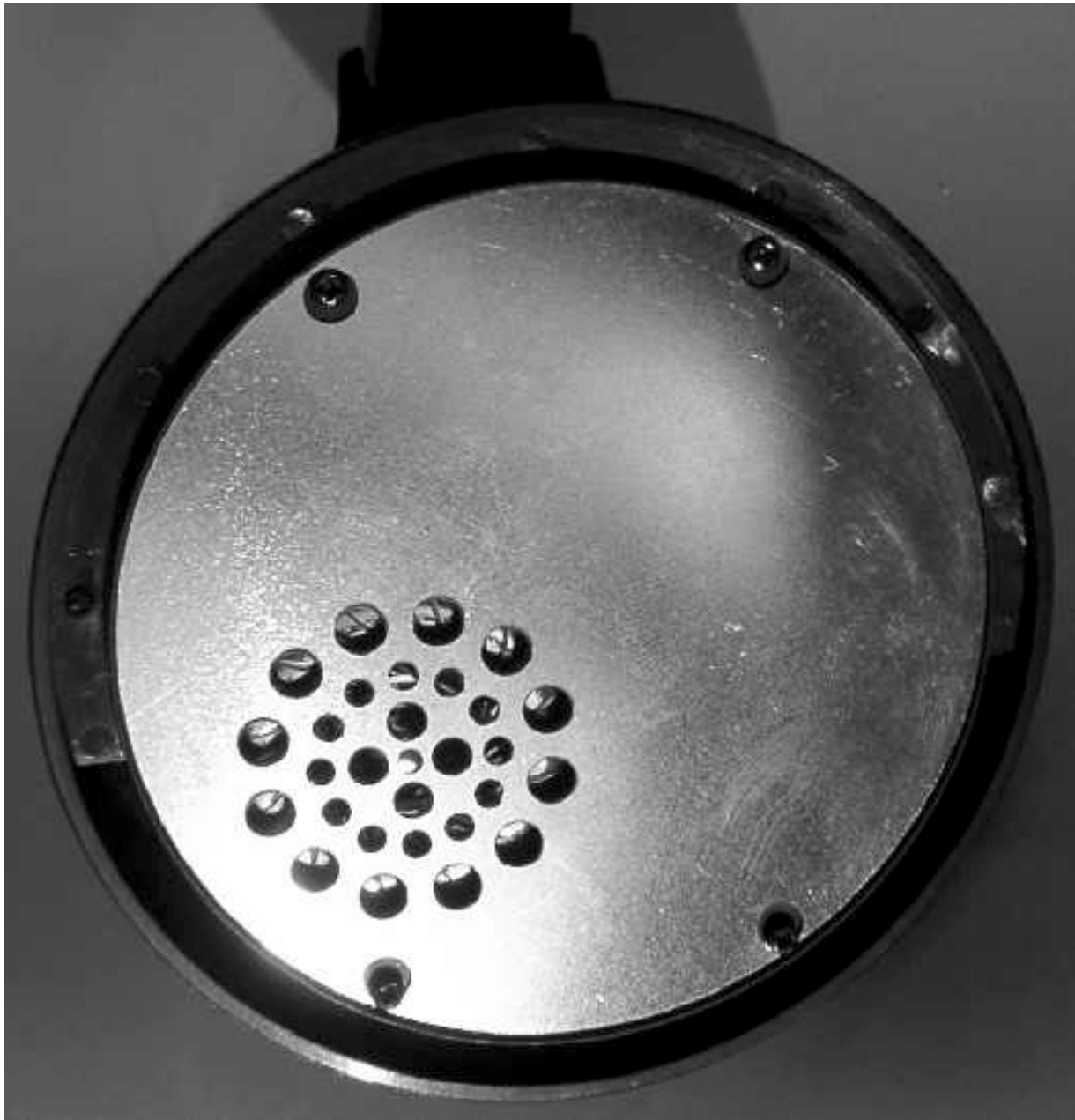
Figure 6: A bufferboard construction of a low magnetic flux H emitting circum-aural stereo headphone for in front localization (de-centric placed speaker, [7]) at right pinna having a MU-metal plated/covered loudspeaker system (see diaphragm plus magnet / coil).
